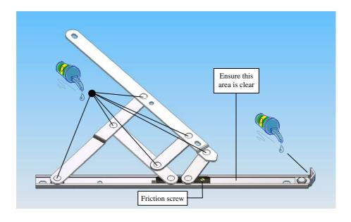
Note: All of the pivot points on a Friction hinge are lubricated during manufacture and should require no further lubrication.
